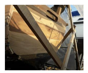
The present owner is carrying out a full restoration. She has had major hull plank repairs, bronze fastened, new transom above waterline, new oak deck beams and a Douglas fir and pitch pine deck. A new Douglas fir mast was completed in 2007.
